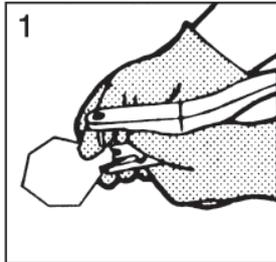
Place the fly tag under the clip by depressing the lever.
