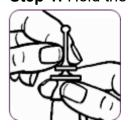
**Step 2:** With the other hand, press downwards on the smaller disk until the 2 disks meet evenly. This will pierce the seal.
