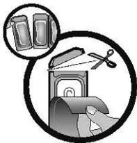
Hold the pipette upright. Tap lightly to ensure the entire liquid content is within the main body of the pipette. Bend the upper border strip backwards. Then the pipette can be set aside, if necessary. To open the pipette, snap off the top of the pipette along the scored line.
