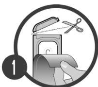
Hold the pipette upright. Tap lightly to ensure the entire liquid content is within the main body of the pipette. Bend the upper border strip backwards. Then the pipette can be set aside, if necessary. To open the pipette, snap off the top of the pipette along the scored line.
