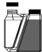
Step 2: Hold the bottle upright and at eye level while slowly and gently squeezing the bottle to fill the dosing chamber to the selected mark.
