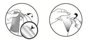
Hold the pipette upright. Tap the narrow part of the pipette to ensure the contents remain within the main body of the pipette. Twist or snap back the tip.
